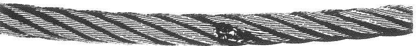
Poor work procedures. Damage to strands and wires resulted from electric arcing.
