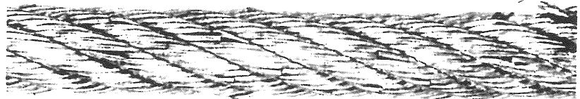
Lack of lubrication. Premature breakage of wires resulted from "locking" of strands, which was caused by insufficient lubrication.
