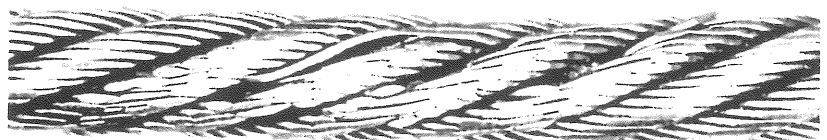
Improper handling. Kink or "dog leg" was caused by improper handling and/or installation. A kink causes excessive localized or spot abrasion.
