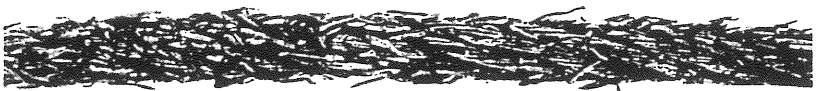
Too long in service. Repeated winding and overwinding of this rope on a drum while it was under heavy stress caused the unusually severe wear shown.
