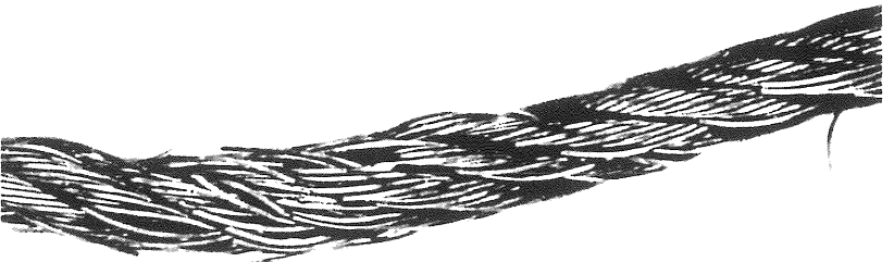
Undersize sheave grooves. Sheaves were too small, causing strands to pinch. Wires then fail in the valley between the strands.
