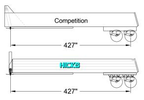
The 93" wide inside width is standard allowing lower sides and CG, therefore increased rigidity.
